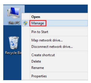
2. Open the Device Manager and go to Network adapters, and then find the corresponding TP-Link adapter, right click it and then go to Properties;
